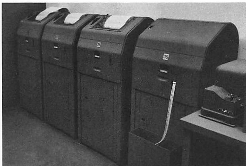
Today's Teletype equipment automatically transmits messages to one or many points at rate of 75 words per minute.
