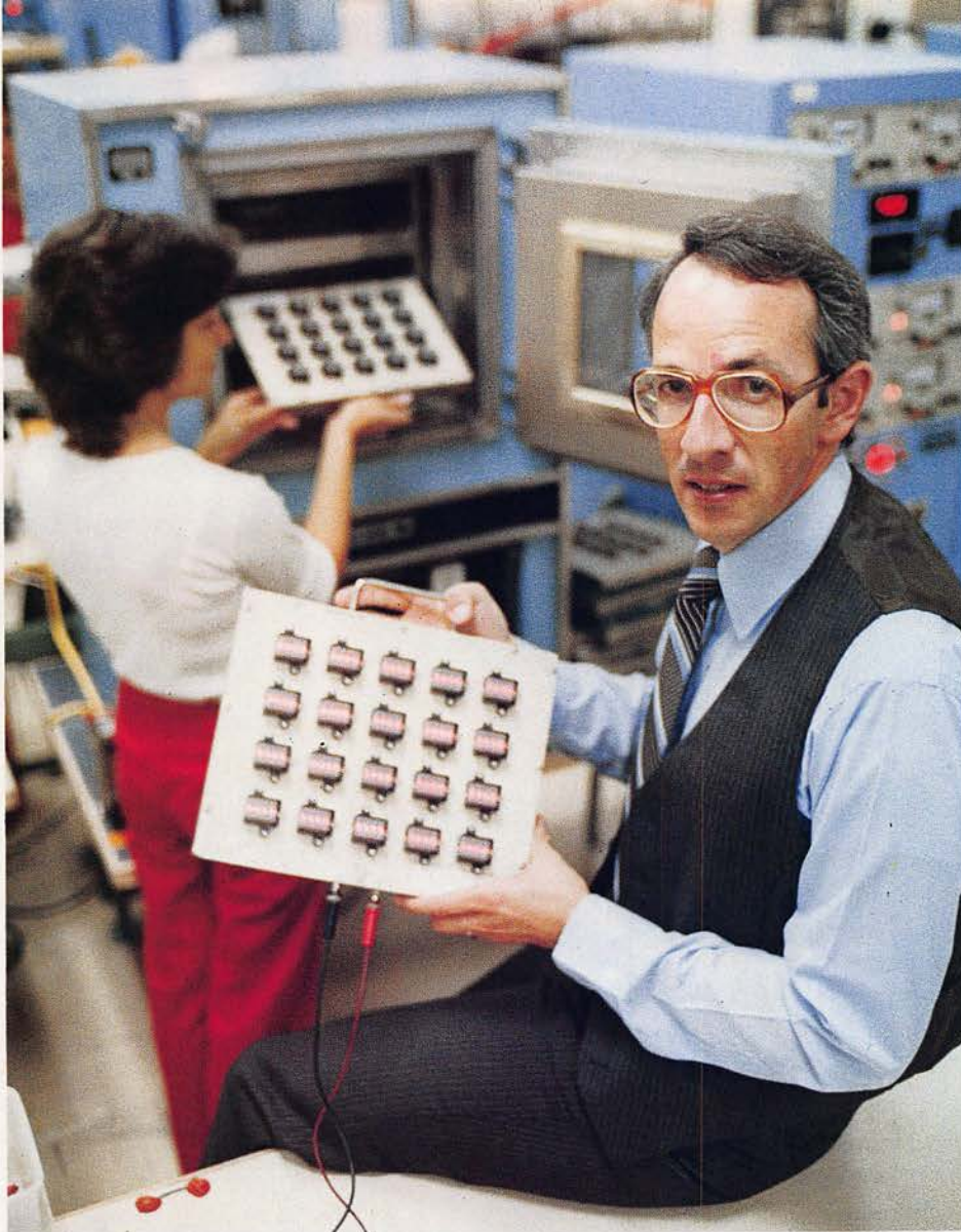
Dan DiLeo holding a rack of light-emitting diodes that are about to undergo a rigorous aging test.
