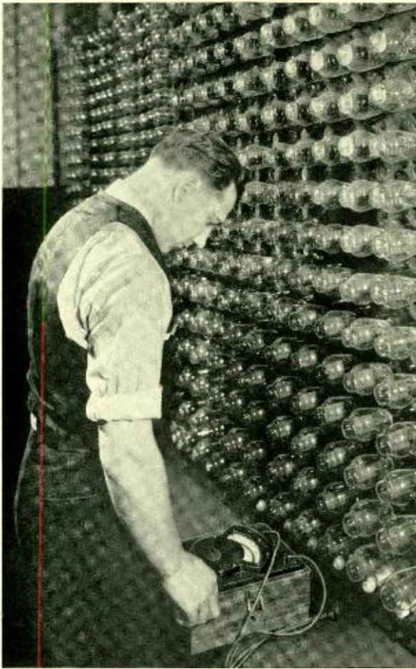
Fig. 5—L. G. Petrovich checking operating conditions of 300A vacuum tubes on life test
